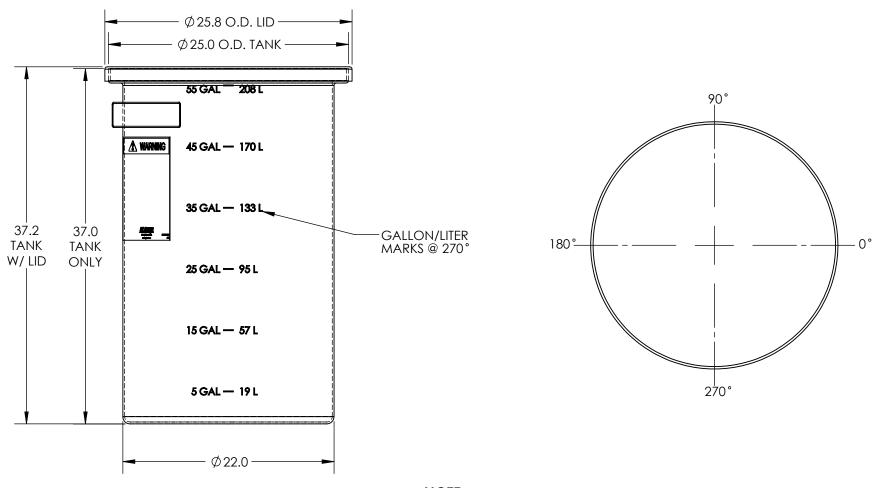
NOTE: TANK CAN BE SOLD WITH OPTIONAL STAND. TANK WITH STAND DRAWING GALLON MARKS CAN BE REMOVED FOR FITTING PLACEMENT AS NEEDED.
